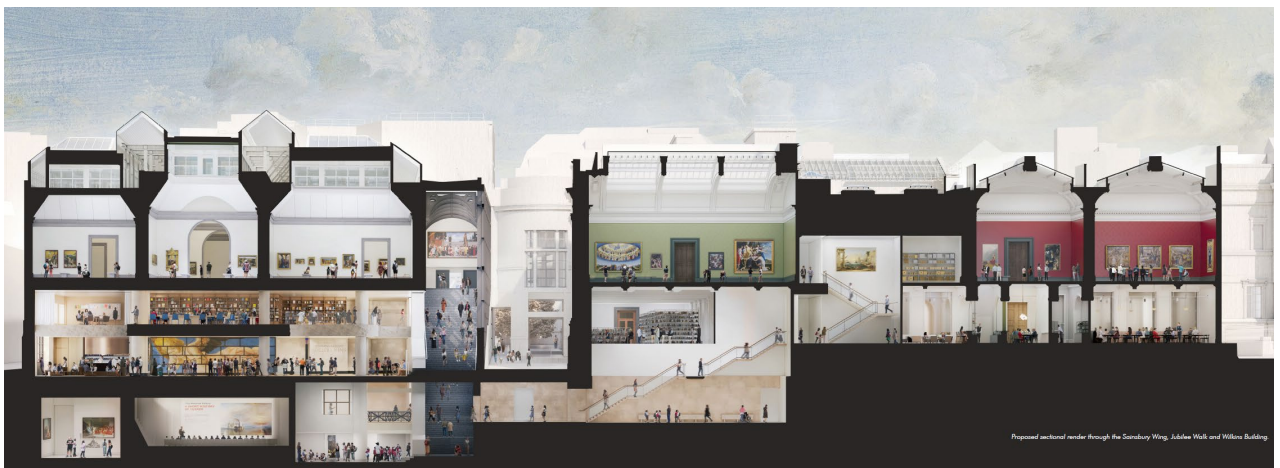
Images of proposed new stair from new basement link into the existing floors of the Wilkins Building
